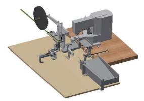
Figure 10. Complete system designed for tie rod cutting
