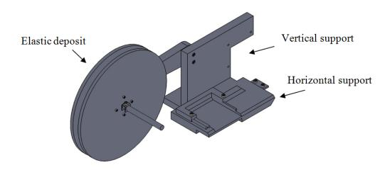
Figure 3. Design of the vertical base part of the automation system
